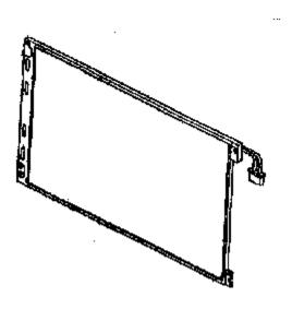
Figure 1-10 LCD module
